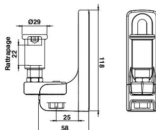
Support aluminium olive de guidage (sans fixation)
