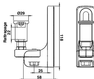
Support zamak olive de guidage (sans fixation)
