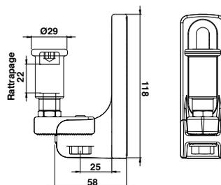
Support aluminium olive de guidage (sans fixation)
